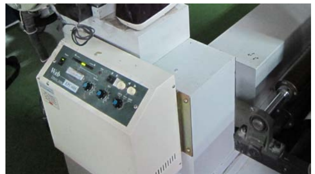
Controller Series 57/68 is installed on Silting Machine by Wall-Mounted
